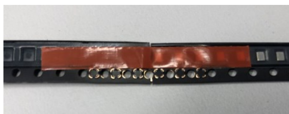
Figure 2 – Cover tape joined using a sticker
