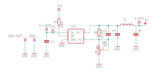
Crystal oscillators are used for frequency control in electronics for many reasons including their very low noise levels. However an oscillator's performance can be significantly degraded by power supply noise. Using low cost switch mode power supplies with internal switching in the kHz range can create frequency distortion on the output of the oscillator.
