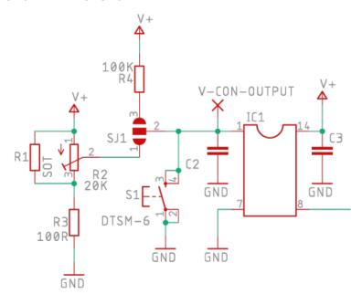
Most SPXO and TCXO products include a function to stop the output of the device by inputting a logic 1 or logic 0 to Pad 1 of the oscillator.
