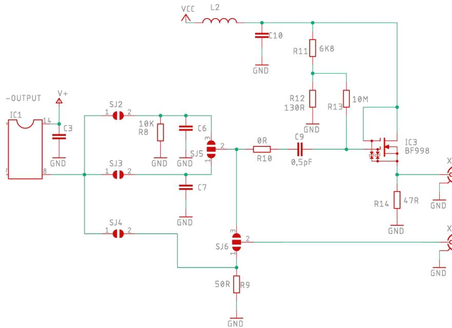
For optimum performance oscillators must have correct loading between the RF output and the input of the following device. Incorrect loading can result in increased current draw within the oscillator which can cause internal heating and thus affect the frequency stability.
