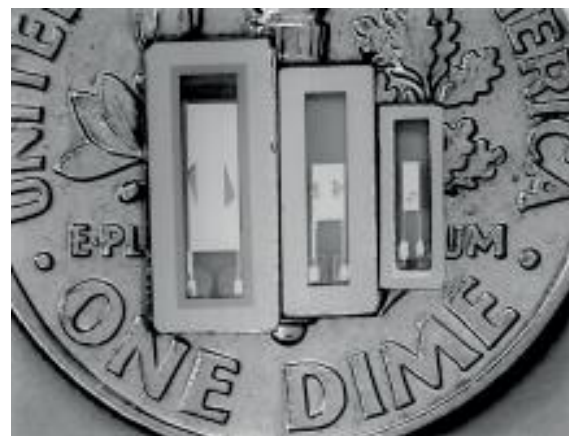
Figure 1: Three AT-strip resonators of three sizes. From left to right: A CX-1, CX-3 and CX-4.
