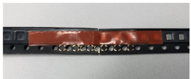
Figure 2 – Cover tape joined using a sticker
