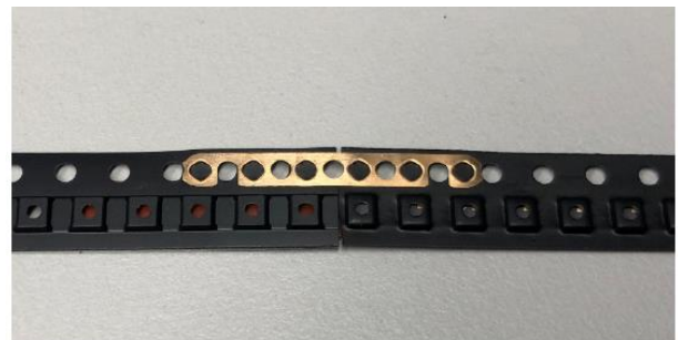
Figure 1 – Tape joined using a metal staple
