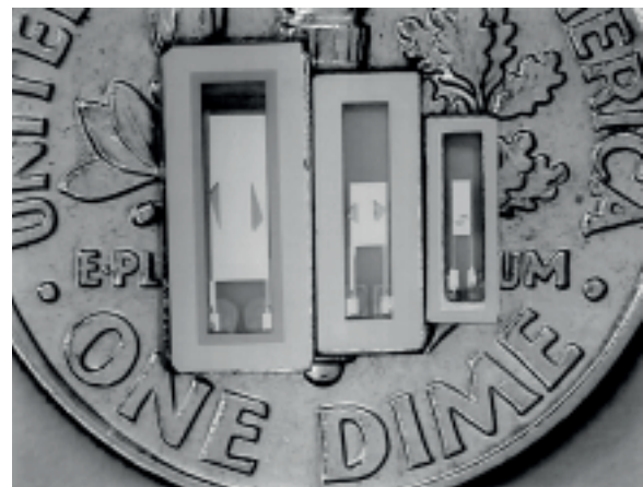
Figure 1: Three AT-strip resonators of three sizes. From left to right: A CX-1 a CX-3, and a CX-4.
