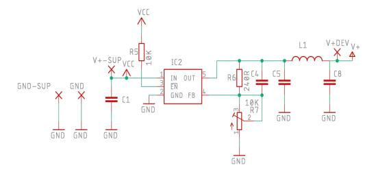
Crystal oscillators are used for frequency control in electronics for many reasons including their very low noise levels. However an oscillator's performance can be significantly degraded by power supply noise. Using low cost switch mode power supplies with internal switching in the kHz range can create frequency distortion on the output of the oscillator.
